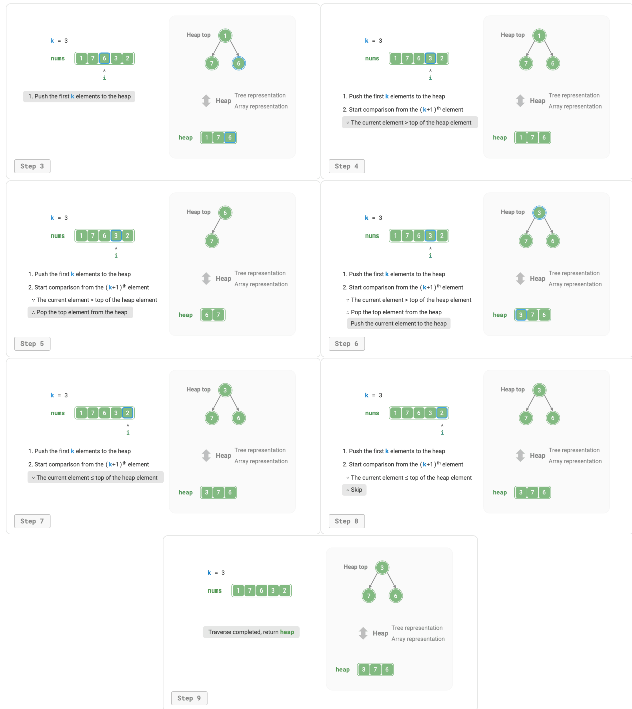
Figure 8-8 Finding the largest k elements using a heap
