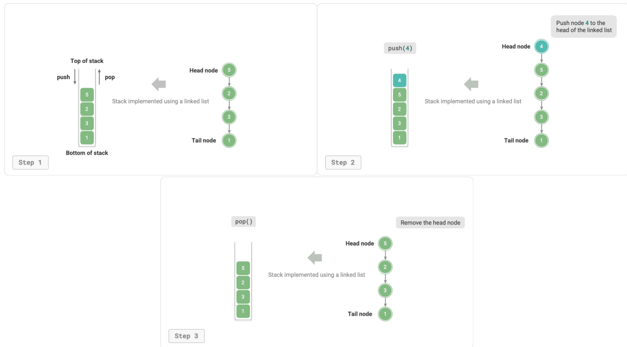
Figure 5-2 Push and pop operations in linked list implementation of stack
