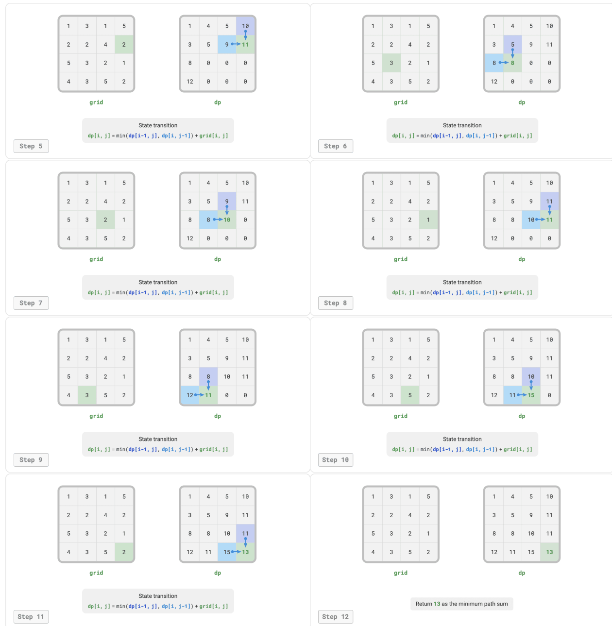
Figure 14-16 Dynamic programming process for minimum path sum
