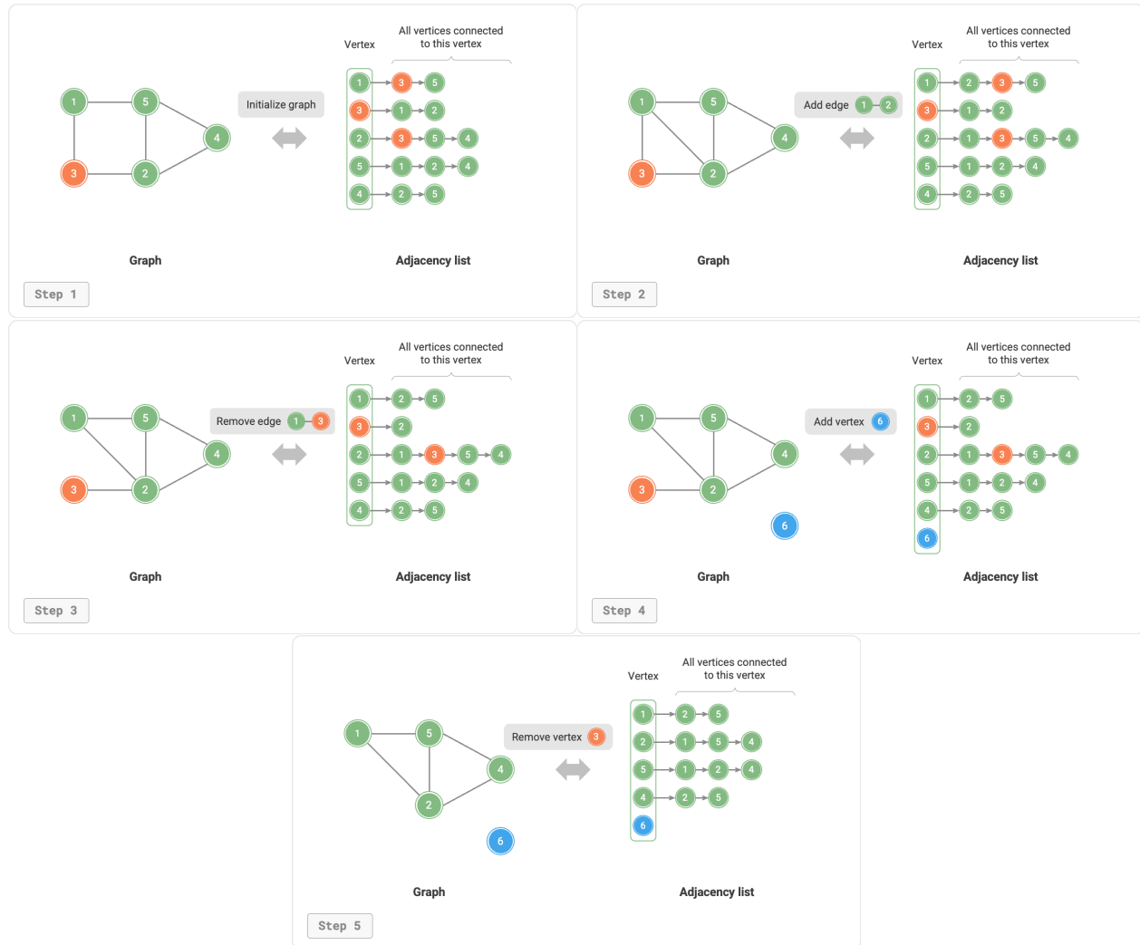
Figure 9-8 Initialization, adding and removing edges, adding and removing vertices in adjacency list
